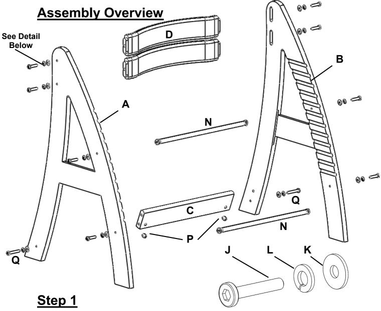
Attach one end of **CONNECTING ROD (N)** into **LEFT** or **RIGHT** side panels (**A** or **B**). Insert the **Screw (J)**, **Spring Lock Washer (L)**, and **Washer (K)** thru the side panel and hand tighten. **NOTE: DO NOT** fully tighten screws at this time.
